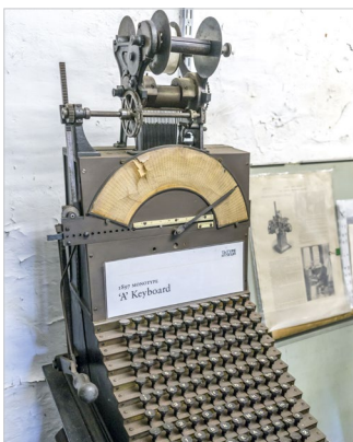
Clockwise from top: Toshi holding a matrix for casting Albertus; a wood-type carving display with a pantograph, templates, and finished wood type; original 1897 "A" Monotype keyboard for composing type; the Monotype leasing library of large-sized matrices for casting.
