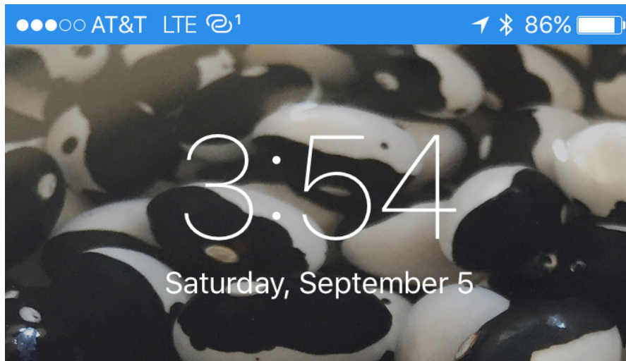
Figure 11: The Lock screen also shows whether the hotspot is active, with a tiny superscript numeral revealing how many clients are connected.
