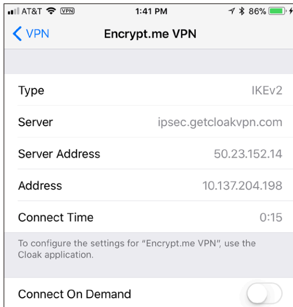
Figure 90: Connection details reveal where the VPN terminates.
