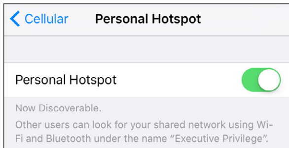
Figure 5: The Personal Hotspot view lets you turn access on or off as well as set a Wi-Fi password.
