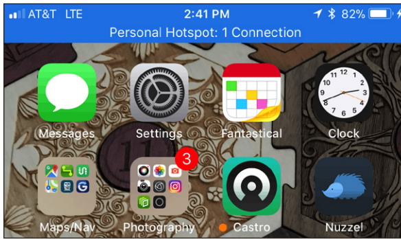
Figure 10: A banner lets you know whenever your device is acting as a cellular modem for a computer via USB, Wi-Fi, or Bluetooth.
